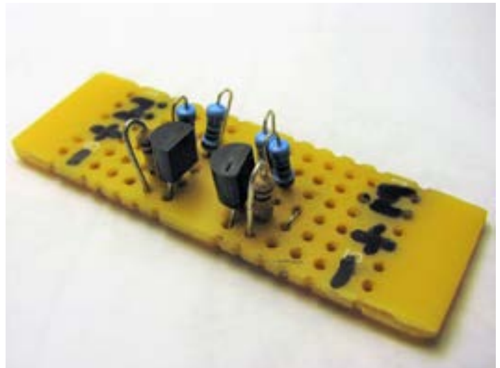
Figure 5. Two limiters on perf board before separation
